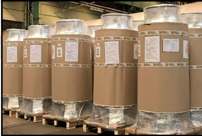
The AC line storage and transport cylinders for liquefied gas represent import components of the Auguste Cryogenics product portfolio. These pressure vessels are manufactured by Auguste Cryogenics in Košice, Slovakia. The trusted products have been successfully operating throughout Europe and all over the world for decades.
