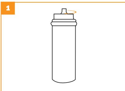
Direct the valve away from you, press it down and turn it clockwise until it is locked.
