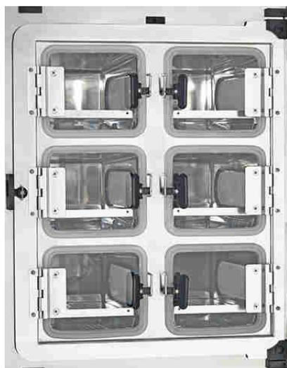
Sixfold gas tight screen for *CELL LOCKER*
