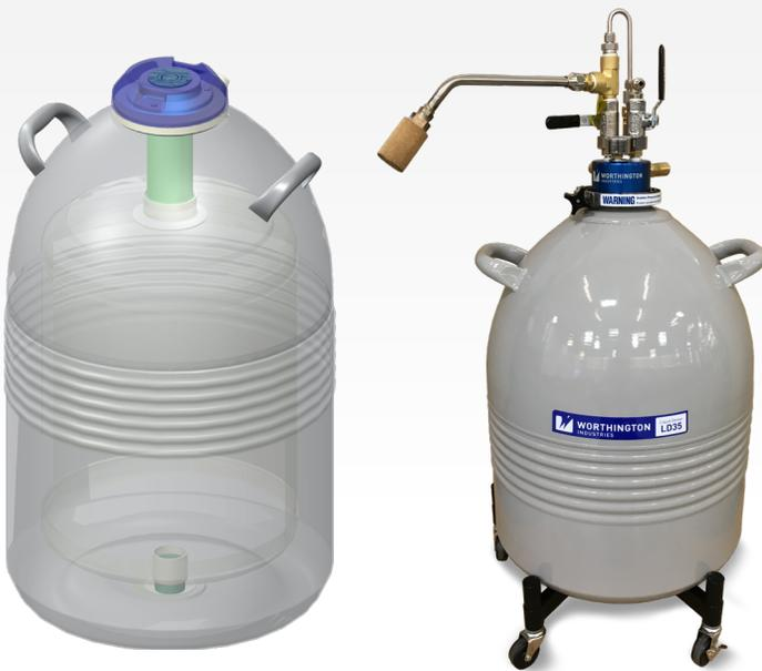
LD35 with Roller Base (P/N 366783) and Liquid Withdrawal Device (P/N 369383).
