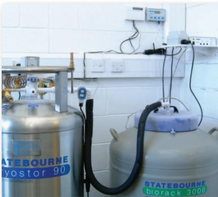
Bio Rack Autofill and Cryostor option (see next page) connected to Data logger low level alarm and autodialler.
