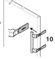
4. Transfer pin on hinge bracket to the opposite side.
