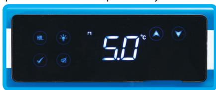
The touch screen controller is completely flat so can be thoroughly cleaned and disinfected as there are no raised buttons to collect dirt and germs. The controller displays, alarms and records minimum and maximum temperatures for both temperature probes. Like a mobile phone touch screen it locks after 30 seconds to ensure that buttons can't be activated accidentally.
