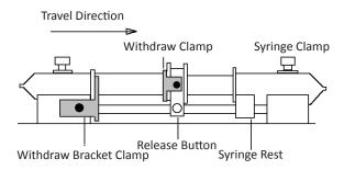
To facilitate loading, the pusher block can be released from the leadscrew by pressing the bronze release button and can be manually moved along the guide rods to accommodate the syringes.
