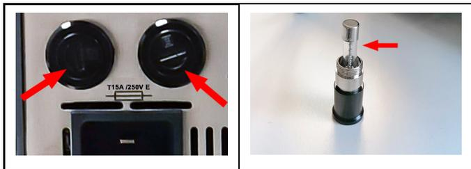
2. Use a flat screwdriver to unscrew the fuse holders [arrows image left].
