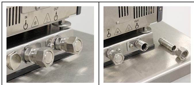
1. Disassemble the union nuts on the pump connectors.
