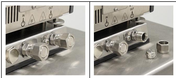
1. Disassemble the union nuts on the pump connectors.
