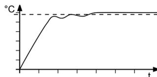
Symptom: Temperature sequence quickly approaches the setpoint, the temperature builds up and the setpoint is exceeded.
