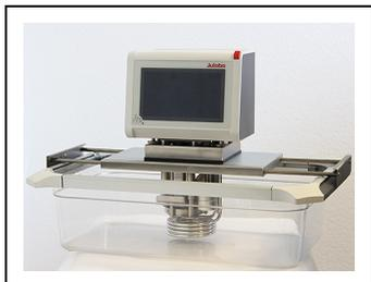
3. Carefully insert the circulator into the bath.
