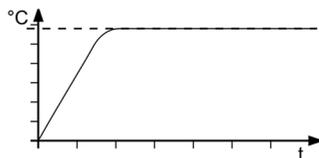
Optimal temperature sequence, temperature quickly reaches the setpoint without overshooting, and keeps the setpoint.
