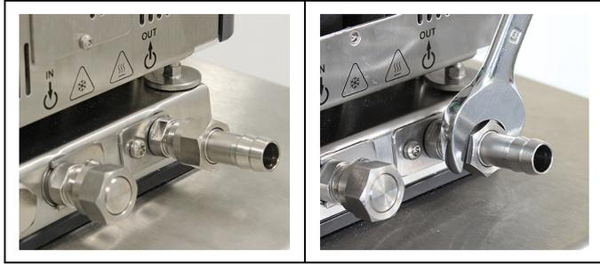
4. Mount the barbed fittings with the union nuts on the pump connections.
