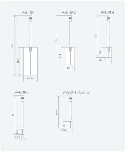
The VAN-SP-4 is specially suitable for testing small-size sample or using sample containers of small openings.
