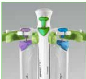
Pipettes can be held in the rubber grips and/or the plunger hooks
