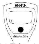
The Checker®Plus features a low battery indicator. When the battery is running low, the tag will appear on screen. When the battery has been depleted, the tag will blink.
