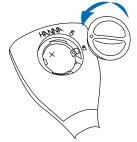
To change the CR2032 Li-ion battery, turn the battery cover located on the back of the meter counterclockwise to unlock. Remove cover and replace with + side facing up.
