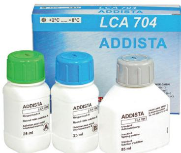
The comprehensive Addista AQA system for Hach LCK cuvette tests contains a standard solution plus two round-robin solutions which allow the user to participate in analysis checking free of charge. Lot number, expiry date and target values by parameter are delivered via RFID tag on the packaging.
