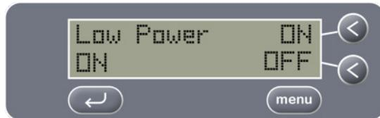
Setting Low Power to ON means that after five minutes of inactivity, the Grant digital ultrasonic bath will enter its SLEEP mode – the screen illumination will power down, and the internal water heater will not operate.
