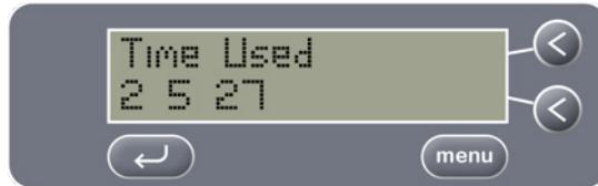
For example, the screen above shows that the bath has been in use for a total of 2 days, 5 hours and 27 minutes.
