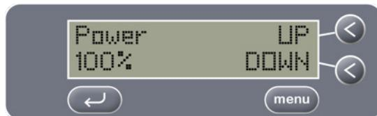
Use the UP and DOWN keys to scroll through the numbers between 50 and 100%. When the desired power level has been selected, use the MENU key to move to the next screen.
