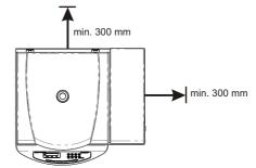
Fig.1 Centrifuge location requirements
