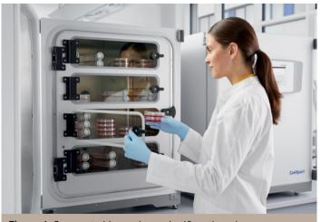
**Figure 6:** Segmented inner doors significantly reduce gas consumption and the risk for contamination.
