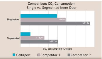
**Figure 4:** The CellXpert significantly reduces gas consumption compared with other  $CO_2$  incubators. Segmented inner doors further reduce consumption (setpoints 5 %  $CO_2$  & 37 °C 3 door openings per day at 5 days a week)
