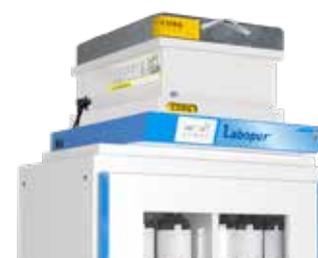
▲ Module with 1 active charcoal filter + 1 security filter
