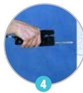
4 Sampling port test of the filter saturation
