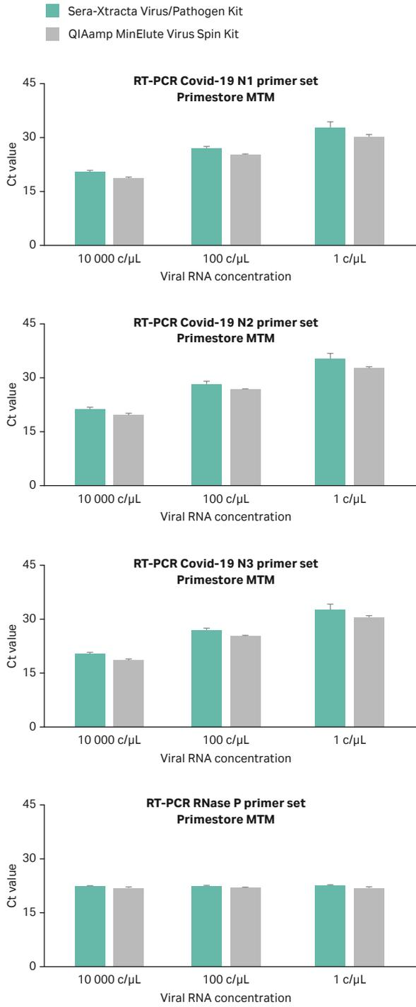
**Fig 4.** Ct values obtained for Sera-Xtracta Virus/Pathogen Kit and QIAamp MinElute Virus Spin kit for varying amounts of the viral synthetic RNA in the input sample as described on the graph. For clarity, Ct values obtained for each of the three SARS-CoV-2 specific primer sets (N1, N2, N3) and human-specific RNase P primer set have been presented in separate graphs. Values averaged from three independent experiments; error bars represent standard deviation.
