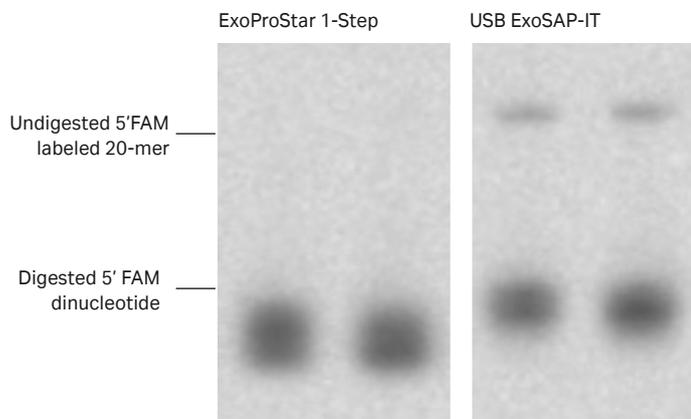
**Fig 2\***. Electrophoretic analysis of the digestion of a 5' FAM labeled 20mer primer. Reactions were conducted according to manufacturer's instructions for ExoProStar 1-Step and USB ExoSAP-IT respectively, using 10 pmol of primer per reaction. No detectable primer remained in the samples digested using ExoProStar 1-Step but undigested primer remained in samples treated with USB ExoSAP-IT.
