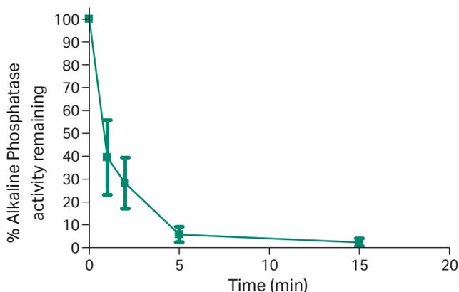
**Fig 5.** Temperature denaturation profile of Amersham Alkaline Phosphatase at 75°C showing rapid and complete denaturation within 15 min. The ExoProStar protocol recommends denaturation of the enzyme components at 80°C, providing even greater confidence in the inactivation of both enzymes prior to further downstream processes.
