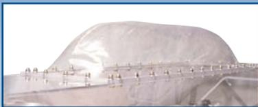
**The Patented Diaphragm Top**, manufactured from durable PVC vinyl, allows easy access into the rigid COY Glove Boxes by expanding and contracting to compensate for changing volume levels caused by hands being inserted into and removed from the glove box. This minimizes gas expelled into the lab atmosphere and increases comfort, as the user no longer has to fight the gloves.
