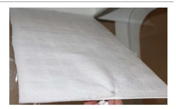
Open the sash and lift pre-filter tray into the inlet cutout. Rotate the wing nuts on each side to support the tray.
