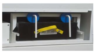
g . Re-install door and lock cam locks using filter door key. The dimples on the locks should be aligned.
