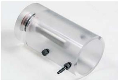
**Cup Horn:** This specialized horn permits high-intensity sound to be applied to multiple samples without direct horn contact. 3.0" diameter only.
