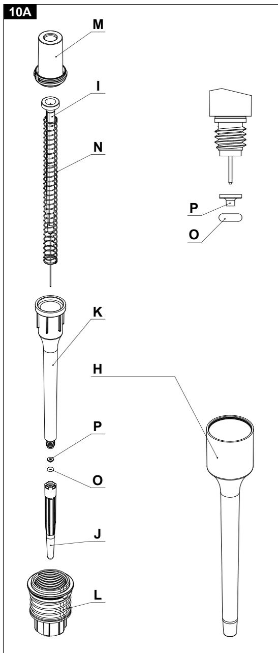
**Single-channel pipettors 0.1-2, 0.5-10, 2-20  $\mu$ L (Figure 10A)**
