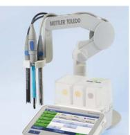
uPlace<sup>™</sup>: the electrode arm can be operated with one hand, moving perfectly straight up and down to bring the electrode to the perfect position. This allows for faster measurements and poses less risk of the sample vessel tipping over and damaging the sensor!
