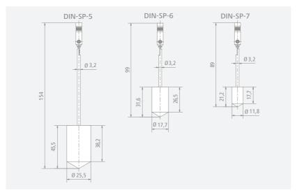
/// Measuring chamber innerdiameters (mm)
