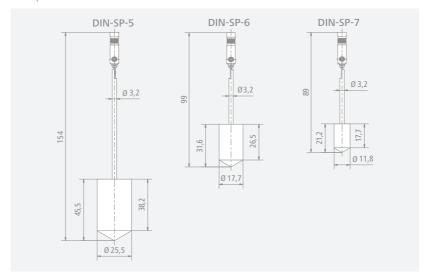
/// Measuring chamber innerdiameters (mm)
